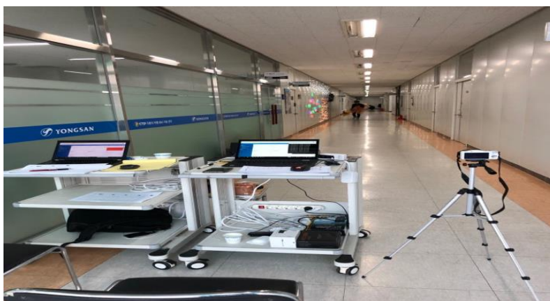
Figure 2. Structure of the testing environment for identifying clutter characteristics.
