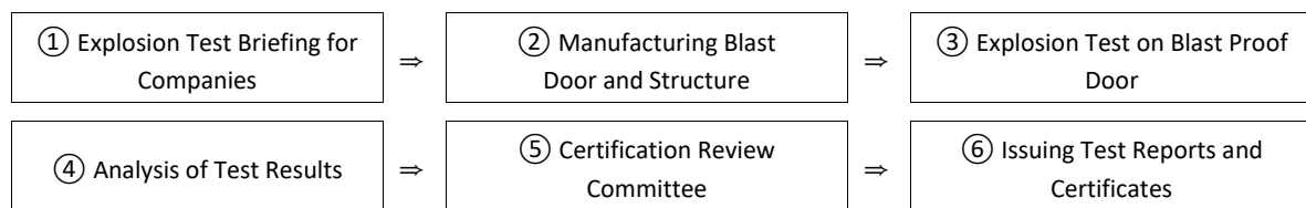
Figure 2. Blast door explosion test certification procedure.
